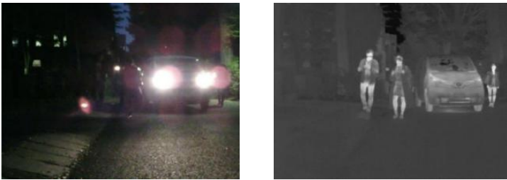
Comparison of RGB- and thermal image in a bright scene
