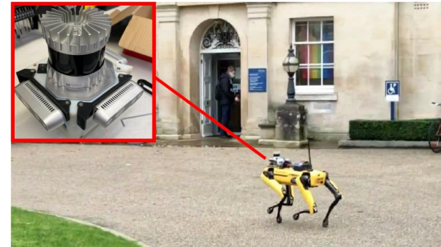
Legged robot scanning a building
